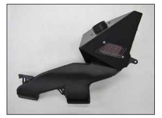
8. Install the AEM® badge into the upper air filter housing and then assemble the two filter housing halves and fresh air scoop and secure with the provided hardware.
