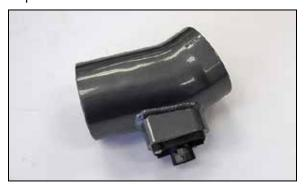
10. Remove the mas air sensor from the factory housing and install it into the AEM® intake tube using the hardware provided.
