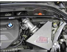
11. Install the provided coupler onto the intake tube but do not secure. Install the intake tube assembly into the factory intake hose and align with the filter adapter, slide the coupler onto the adapter and adjust the assembly for best fit. Secure the intake tube assembly with the provided hose clamps. Reconnect the mass air sensor electrical connection.
