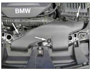
3. Remove the two bolts that secure the fresh air intake duct too the core support. Release the locking tab at the air filter housing and then remove the fresh air intake duct.
